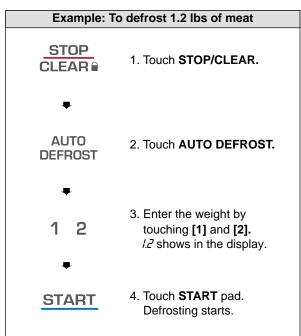
The display changes to defrost time count down. The oven will beep during the DEFROST cycle. At this time, open the door and turn, separate or rearrange the food. Remove any portions that have thawed. Return frozen portions to the oven and touch START to resume the defrost cycle. The oven will not STOP during the BEEP unless the door is opened.
